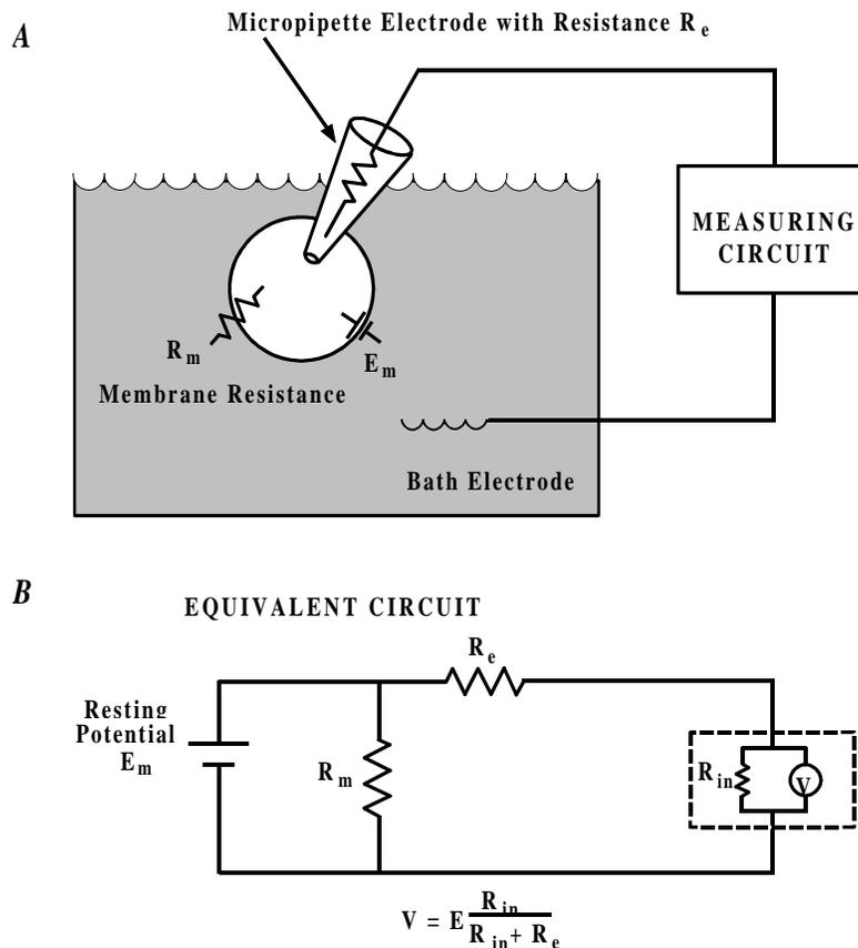
**Figure 1-8.** Representative Voltmeter with Infinite Resistance
