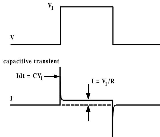
**Figure 1-15.** Typical Voltage-Clamp Experiment
