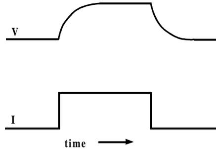
**Figure 1-14.** RC Parallel Circuit Response
